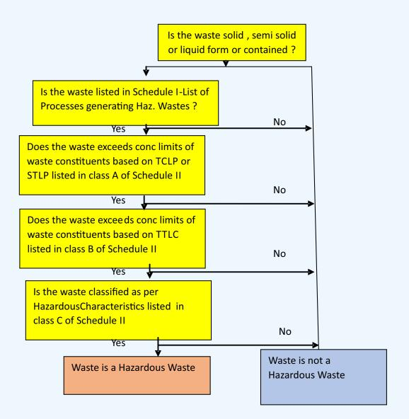
Figure 2.1: Flowchart for determination of hazardous waste as per Rules 2016
