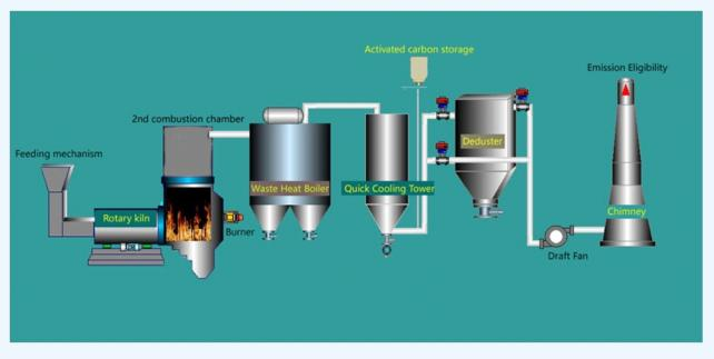
Figure – 7.2.3: Incineration Flow Diagram
